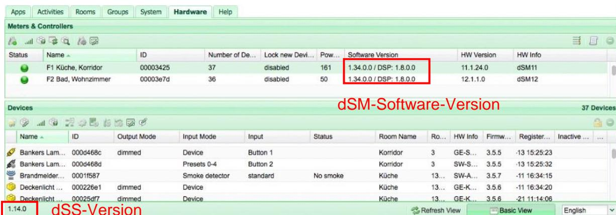
The screenshot shows the 'Hardware' tab in the Digital Strom configurator. It displays two sections: 'Meters & Controllers' and 'Devices'.
