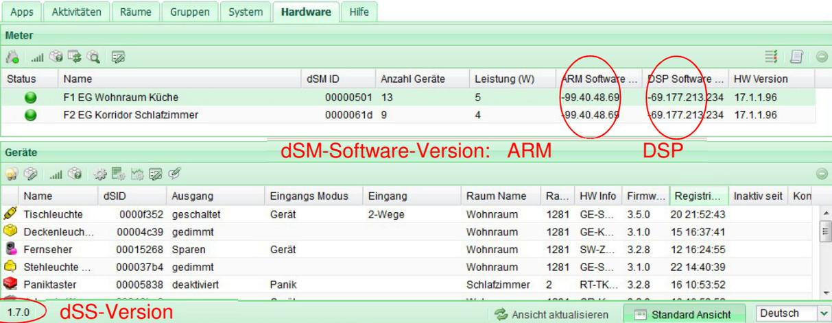
The screenshot shows the 'Hardware' tab of the digitalSTROM configurator. It displays a 'Meter' section with a table of installed meters and a 'Geräte' (Devices) section. The 'dSM-Software-Version' is shown as 'ARM' and 'DSP'. The 'dSS-Version' is highlighted as '1.7.0'.
